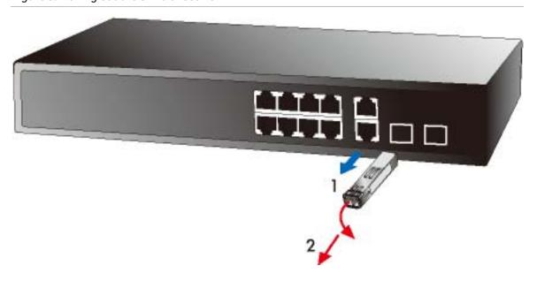
**CAUTION:** Never pull out the module without pull the handle or the push bolts on the module. Pulling out the module with too much force could damage the module and SFP module slot of the Managed Industrial Switch.
